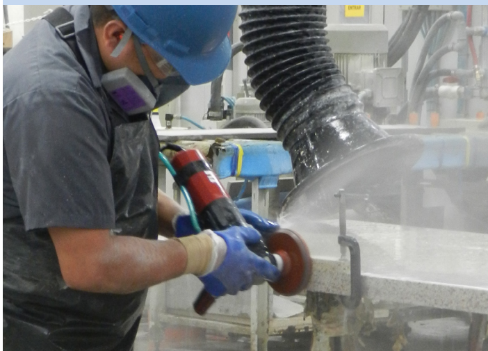
Water and dust-capture systems can decrease dust levels.
